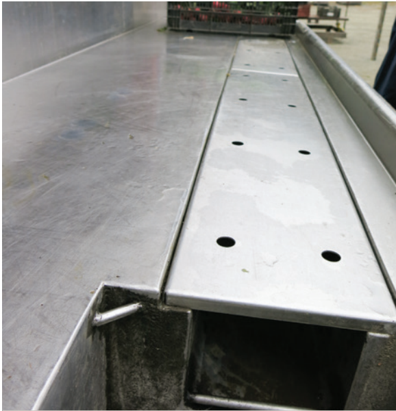
Stainless steel spray tables like this one with a channel for spray water to drain off are sometimes available when restaurants go out of business. Tianna DuPont, Penn State Extension
