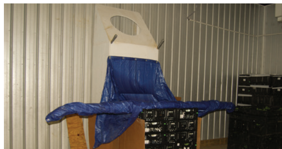
Clean baby greens are cooled by forced-air cooling inside a larger walk-in. Andy Andrews, Spiral Path Farm
