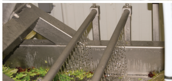
In this hydrocooling system, lettuce on a conveyor goes through chilled (34°F) water in order to quickly cool. Andy Andrews, Spiral Path Farm
