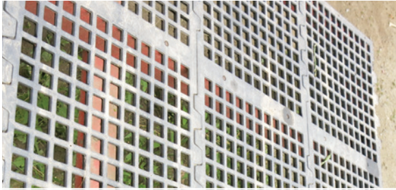
Spray tables made with floor tiles provide an easily cleanable surface that is also smooth and less likely to nick produce. Tianna DuPont, Penn State Extension
