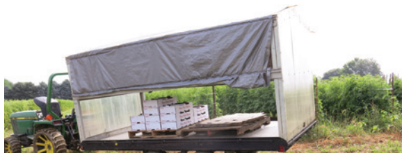
Canopies on harvest trailers help keep produce cool and keep birds from contaminating produce. Tianna DuPont, Penn State Extension
